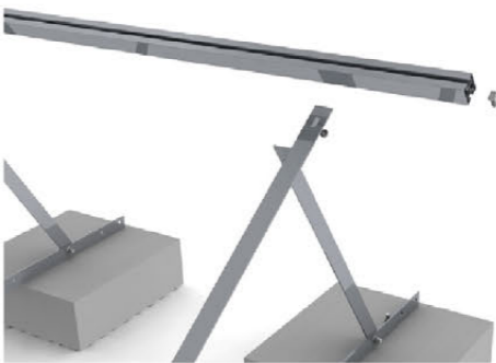
2 Fix the rail on the triangular supporting frames with T-head bolt and flange nut.
