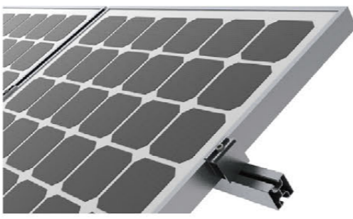
3 Insert the end clamp and middle clamp into the slot of the rail. Then put the PV module onto the rail, and fasten the inner hex bolt to fix it.
